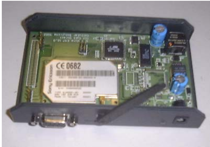
UltraLite Intelligent Terminal internal view
